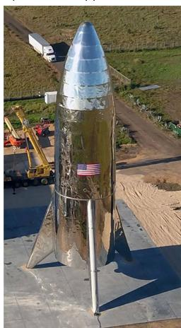
SpaceX is building a test article dubbed "StarHopper" for its proposed two-stage reusable spaceship dubbed the "Starship."
